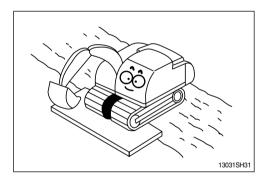
When operating in water or when crossing shallow, check the bed soil condition and depth and flow speed of water, then proceed taking care that water is not above carrier roller.
