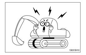
Operate carefully to make sure all personnel or obstacles are clear within the working range of the machine.
